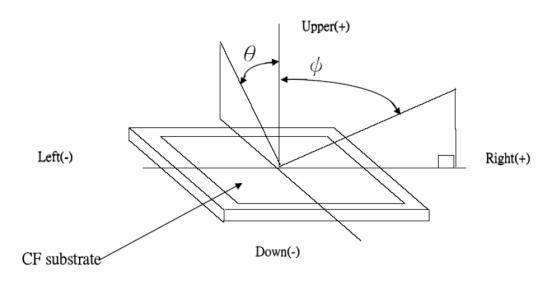
Fig.1 Definition of Viewing Angle
